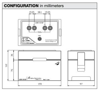
The resistive elements are held by special designed case so, it's suitable for environment with vibration during transportation.
