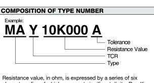
characters, five of which represent significant digits. R or K is a dual-purpose letter that designates both the value range (R for ohmic; K for kilo-ohm) and the location of decimal point.
