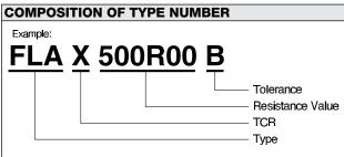
Resistance value, in ohm, is expressed by a series of six characters, five of which represent significant digits. R or K is a dual-purpose letter that designates both the value range (R for ohmic; K for kilo-ohm) and the location of decimal point.
