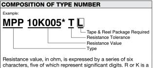
characters, five of which represent significant digits. R or K is a dual-purpose letter that designates both the value range (R for ohmic; K for kilo-ohm) and the location of the decimal point.
