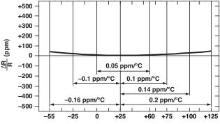
Ambient Temperature (°C) and TCR Chord Slopes for Different Temperature Ranges
